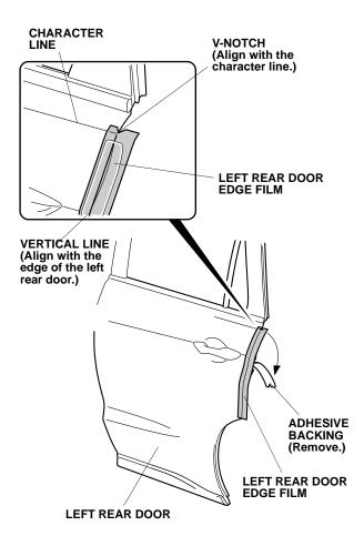
19. Align the vertical line on the left rear door edge film to the edge of the left rear door. While applying light pressure, carefully remove the adhesive backing.
